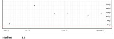
Dissolved oxygen concentrations are measured using either a YSI probe or a Hach kit with a drop-by-drop titration to show a change in water colour until totally clear. Red line indicates the Environmental Quality Guidelines for Alberta Surface Waters (2018) for exceedance is minimum 5 mg/L for instantaneous value.
