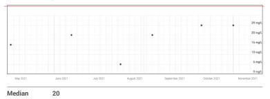
Chloride concentrations are measured using Hach kits with a drop-by-drop titration to show a change in water colour from yellow to orange. Red line indicates the Environmental Quality Guidelines for Alberta Surface Waters (2018) for exceedance is maximum 120 mg/L.
